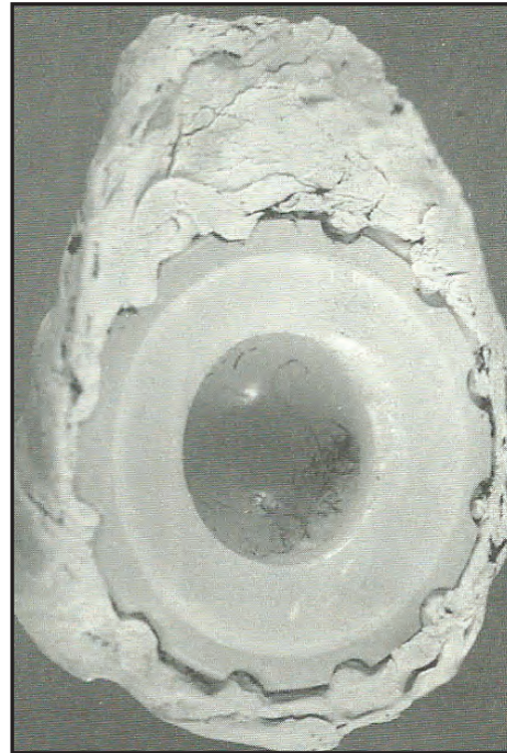
Fig. 5. Retrieval of Charnley acetabular component with metal cable debris embedded in its articular surface. 6
