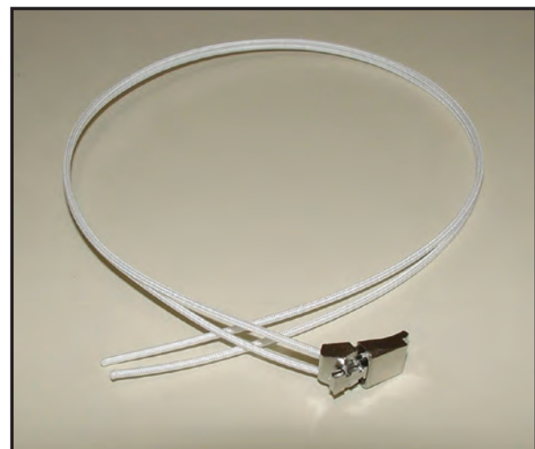
Fig. 3. Polymer SuperCable comprised of UHMWPe fiber and nylon filament with a titanium locking clasp.
